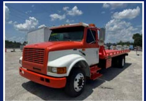
'99 Roll Back 4700 DT466E -191,173 mi, 212 wheel base, air brakes, Century 21' steel bed, 8K Ramsey winch, brand new tires all the way around. \$19,900 OBO
