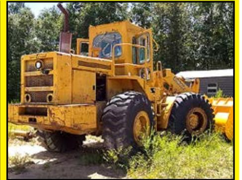
'93 Kawasaki 80Z11 - Runs OK, 8.3 turbo Cummins turbo diesel, 6CT engine, many parts available.
