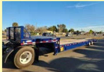
**Q26449 - '16 Ledwell LW48 HT2-10-PB-LP 48' x 102" Lowboy Trailer, 40 ton capacity, hydraulic beaver tail & front ramp, hydraulic winch, Air-Ride suspension, steel wheels, 235-75R17.5 tires. **\$45,900.****
