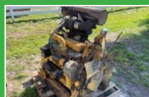
John Deere 4045 - 4 cyl. diesel turbo engine, twin disc, C110HP4 power take off. $6,500.
