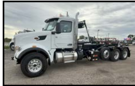
'26 PETERBILT 567 - X15 Cummins 500Hp, Allison 4500, Steerable Lift Axle, Haulmaxx Suspension, Galfab Hoist, Pioneer Tarp. $269,500.
