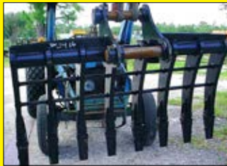
NEW Mini Excavator Rake 48" - fits CAT 307 & 308, 50mm pins, 7.5" between ears, tines 24", wt. 152#. $1600.
