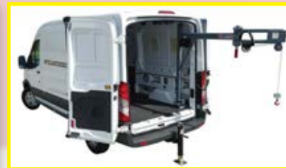
Venturo Van Crane - 1,000 lb cap., 6K ft-lb rating, 6' ext. boom reach, 4'6" stowed, 220 lb unit, 12VDC winch, 1.3 HP motor, 25.5 FPM line speed. $3,500 installed.
