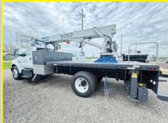
New Ford F750 - Non CDL, Manitek SC-62, 6k lbs. load line, 62' working height, new w/ warranty. $299,900.
