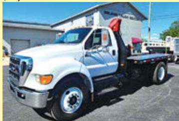
Q26423A - '15 Ford F750XL Custom Hauler w/ Fassi F50 knuckle boom crane, 6.7L Cummins 260HP, Allison auto, A/C, 185K mi., P/W, P/L, gooseneck & pintle/ball hitch, airbrakes, 11R22.5 tires, 33K GVW $41,900.
