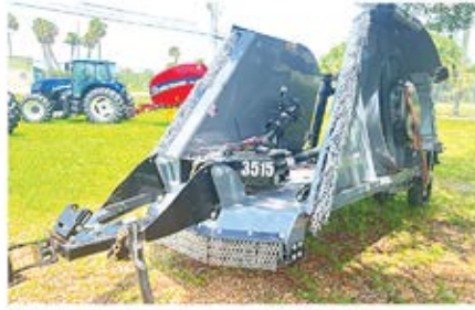
3515 15' Flex wing cutter min. PTO 60 HP, 10 gauge gear box, 235 hp splitter box, outboard gear box, 190hp.
