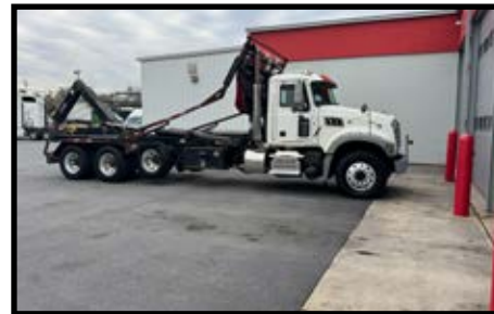
'20 Mack Granite - MP8, Allison 4500, Tri Axle, Camelback Suspension, 300K mi. $149,500.
