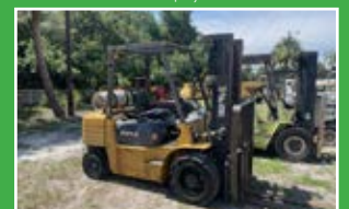
CAT GP30 - 4 cyl Mitsubishi engine, 3 stage w/ side shift, 5800 lbs lift cap, 3365 hrs. $10,500.
