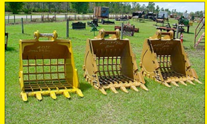
Skeleton Excavator Buckets - 80mm pins, overall width 48", CAT320. 3 available. $4,200 each.
