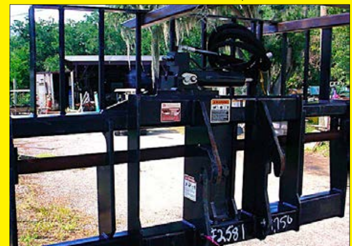
LIKE NEW JCB Telehandler QC Hydraulic Tilt Frame - without forks. 6'W. Hook 13-1/2" ctr to ctr. Top pin 2-1/4". Top to bottom ctc 10-1/2". 2-1/4" rod diameter. Fits most telehandlers, including JLG & Genie. $1,750.
