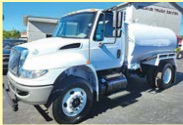
Q26426 - '18 International 4300 Ledwell 2,000 Gallon Water Truck - 6.7L Cummins 200HP, automatic, A/C, 37K miles, air brakes, 11R22.5 tires, 33,000# GVW. $67,900.
