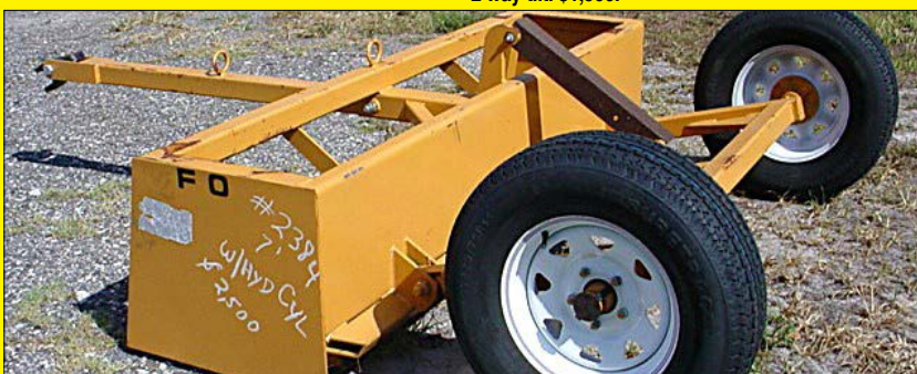
NEW 7' Hydraulic Box Blade w/ hoses and cylinder. Industrias America. $2,500. (8' also available.)
