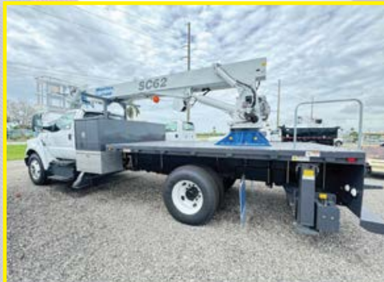
New Ford F750 - Non CDL, Manitex SC-62, 6k lbs. load line, 62' working height, new w/ warranty. $299,900.
