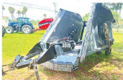
3515 15' Flex wing cutter min. PTO 60 HP, 10 gauge gear box, 235 hp splitter box, outboard gear box, 190hp.
