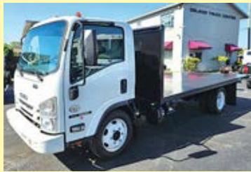
Q26390 - '21 Isuzu NQR - 16' Steel Flatbed, 5.2L Diesel 215HP, Auto, A/C, 77K miles, P/W, P/L, cruise, 225-70R19.5 tires, 17,950# GVW. $45,900.
